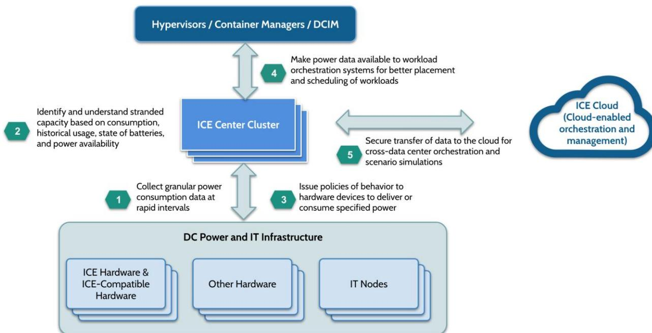
**Figure 1: Software-Defined Power Platform**
