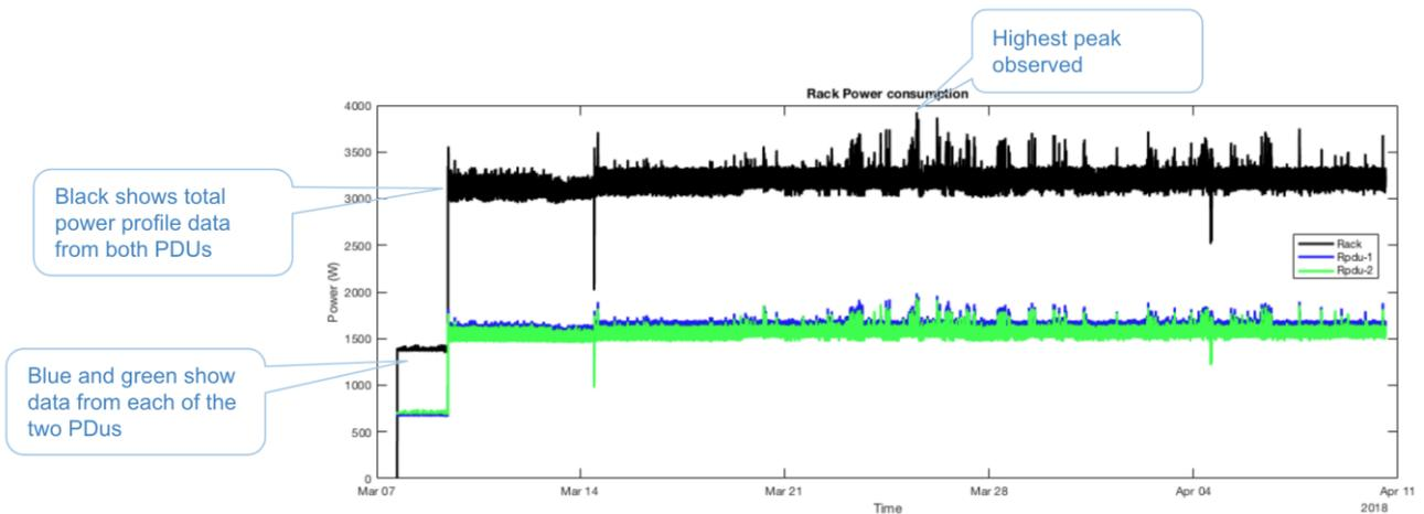
**Figure 2: Power Data Collected Over One Month for One SAP HANA® Rack**
